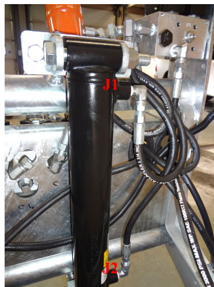
Jack hose installation (18" hoses)
