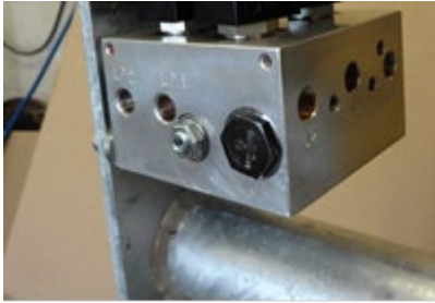
Manifold Installation- front view.
